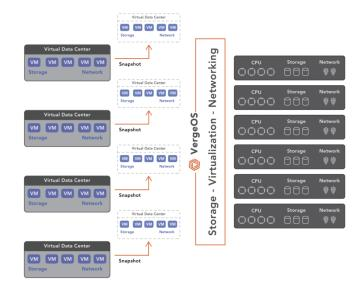
With VergeFabric and VDCs, IT teams gain unparalleled control over workload isolation, network automation, and security enforcement, all without additional licensing fees or complex configurations.
